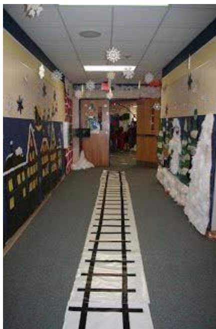
A hazardous amount of combustibles
